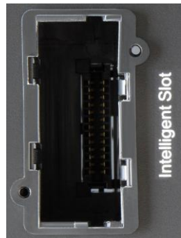
Fig. 3-14 Intelligent expansion slot for the MKD RT series.
