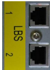
Fig. 3-33 LBS ports 1 and 2 on the rear side of the UPS system.
