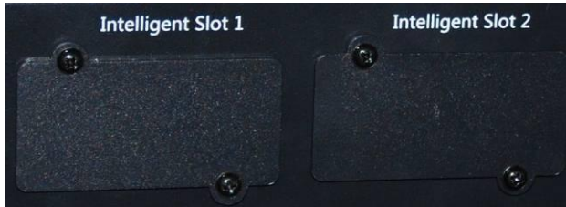
Fig. 3-23 Adapter slots for the accommodation of intelligent extension cards (System variants 30 / 40 and 60 / 80 kVA).
